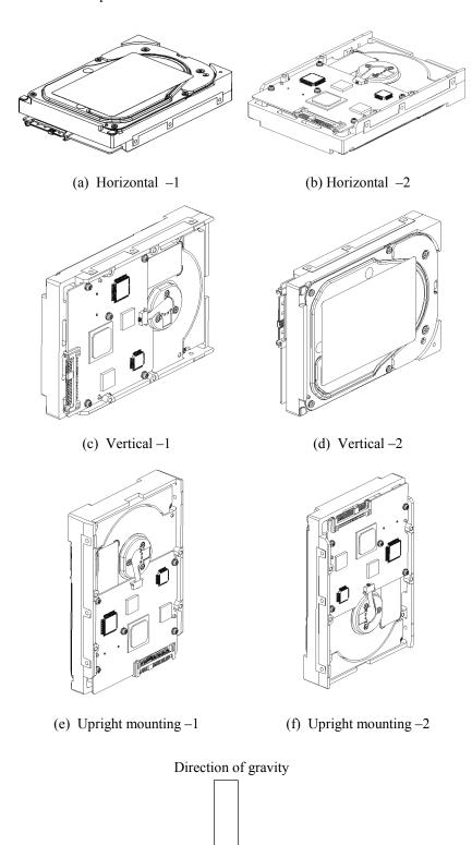
Figure 4.2 HDD orientations
